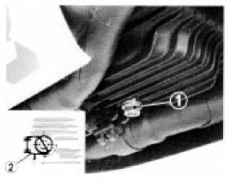
(1) Drain plug (2) Lock wire **ENGINE OIL CHANGE**
