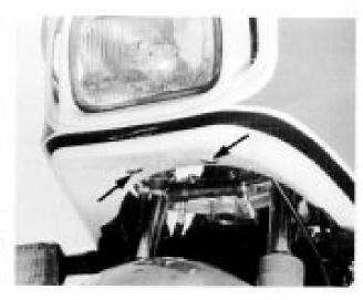
4. Remove the two fairing attaching bolts and remove the fairing from the bracket.
