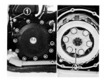
(1) Clutch cable (2) Lifter plate
