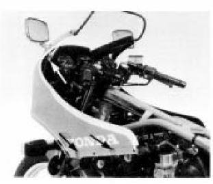
3. Remove the six fairing attaching nuts.
