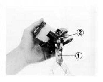
(1) 6 mm bolt (2) Pad pin retainer
