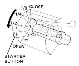
7. When engine rpm begins to pick up, operate the choke knob to keep fast idle at  $1,600-2,000 \text{ min}^{-1}$  (rpm). To speed warm up, open and close the throttle, keeping engine rpm below 2,000. Continue warming up the engine by opening and closing the throttle until it will idle (1,000 min-1) \* Never run the engine in a closed area. (rpm) smoothly.
