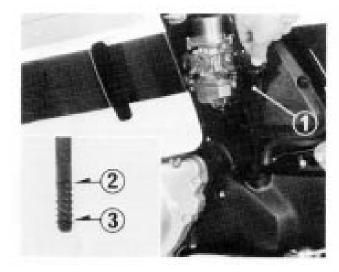
(1) Filler cap/dipstick (2) Upper level mark (3) Lower level mark
